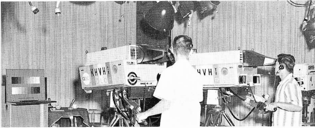
FIG. 5. KVVH-TV technical director Joe Kim and crew chief Paul Hirata aligning TK-42 cameras before "Conversation," a weekly program feature hosted by KVVH Women's Editor, Betty Smyser.
