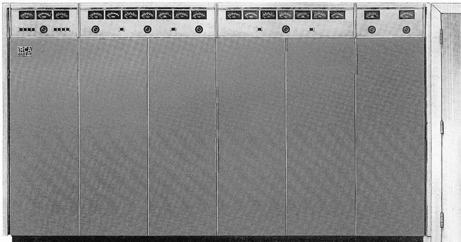
FIG. 1. Parallel Transmitter Installation, using two TT-12EL 12.5 kW TV Transmitters.
