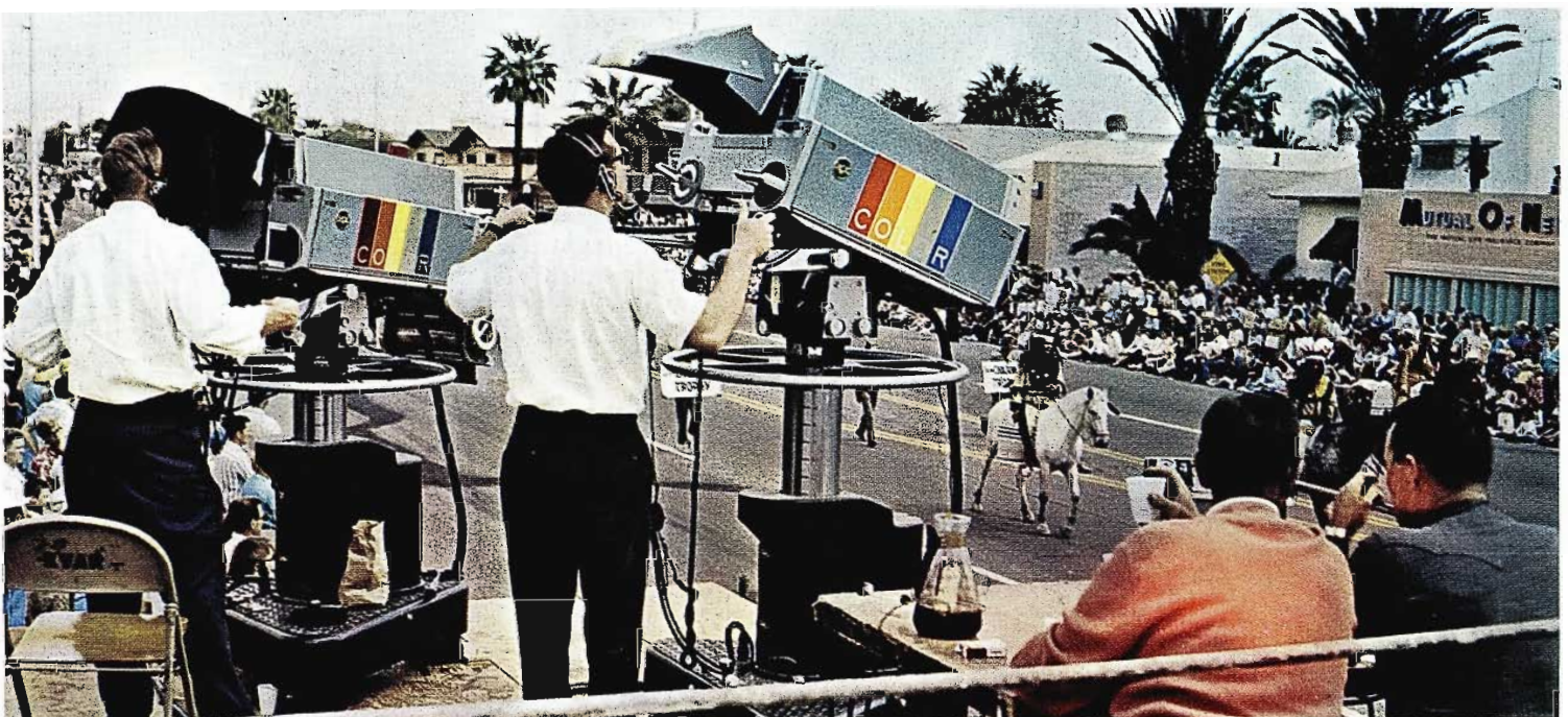
FIG. 6. Because the parade passed close by KTAR studios, it was only necessary to use some 300 foot of cable, a raised 18 ft. platform and a forklift to capture the entire rodeo.
